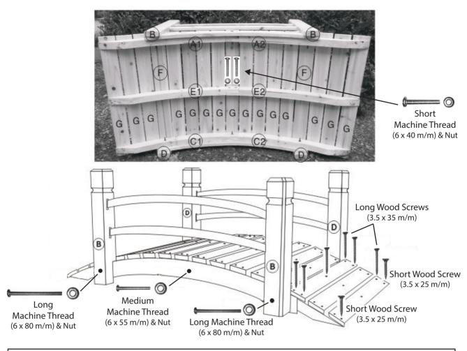
**Step 1**: Connect (A1) to (A2) by overlapping the pieces. Match the hole to the center of (B) rail and use 1pc of Medium Machine Thread (6 x 55m/m) + 1pc Nut. Continue to attach (B) rail at the posts using 2pcs of Long Machine Thread (6 x 80m/m) + 2pc Nuts.
